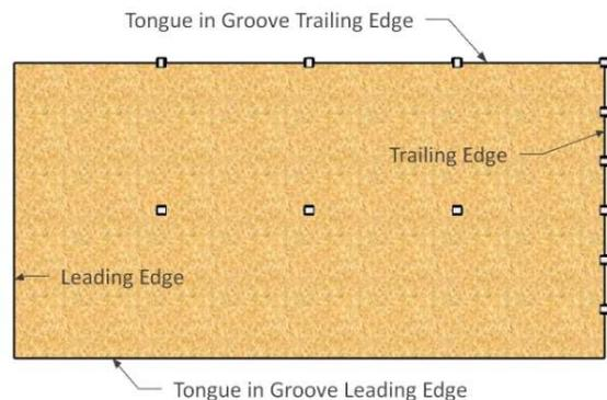
7. Flip panels into position with leading edge down so overlapping pads do not dislodge.
