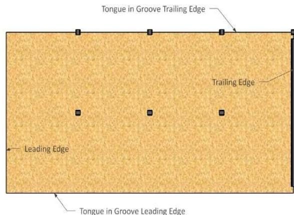
Figure 2: Two-sided tongue-in-groove with strip
